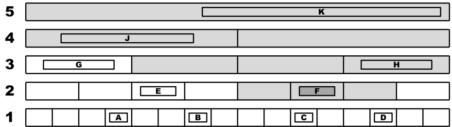
(b) When object F is processed, it is checked against the objects H, J, and K. However, F is not tested against object C since grid 1 possesses smaller cells than grid 2 and thus the intersection between C and F is already found when C is processed.
